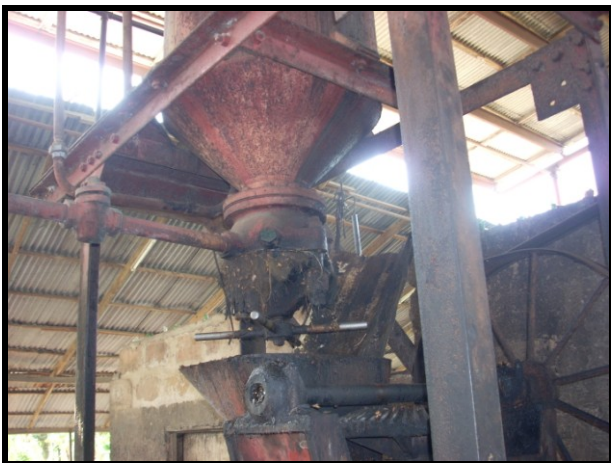
Simple fruit threshing machine used by the mill in Abia State, Nigeria
